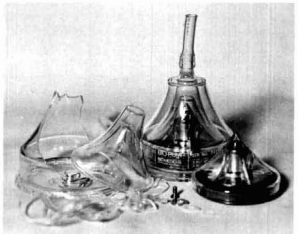
The Bio-Pump after applying a hammer to break the plastic outer shell, left. A complete instrument before destruction is shown at center. At right is the inner plastic container that houses the magnet.
